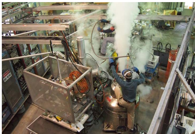
Fig.2: BNL TEBIS with installed \text{HEC}^2 electron gun being prepared for the operation.
