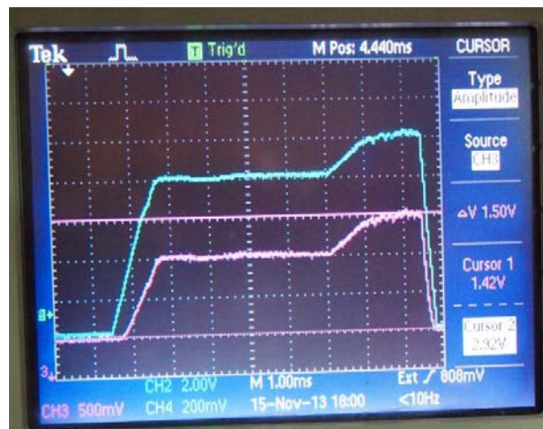
Fig.3: A 7 ms current pulse of at maximum 1.5 A (pink) extracted from the \text{HEC}^2 gun.
