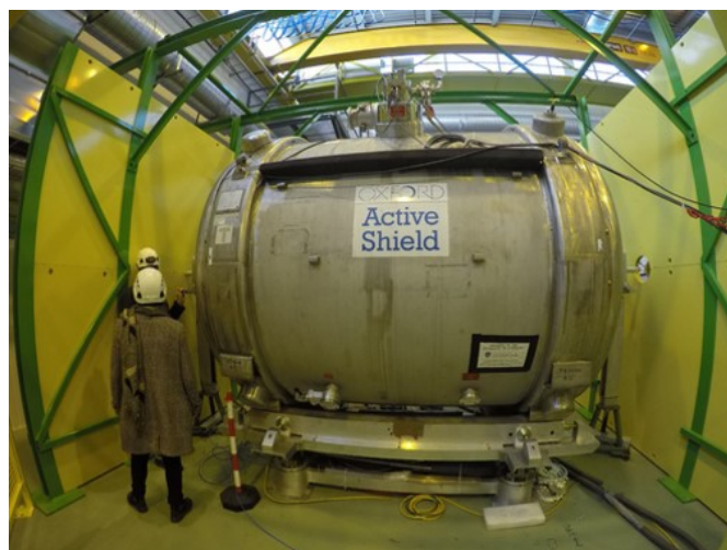
Figure 1: Photograph showing the ISS magnet inside its magnetic shielding.
