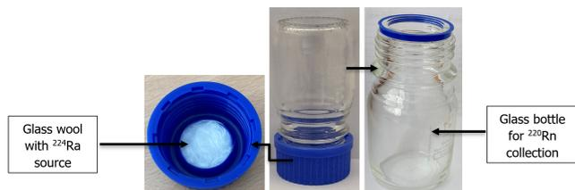
Figure 3:  $^{224}\text{Ra}/^{212}\text{Pb}$  generator by gas collection
