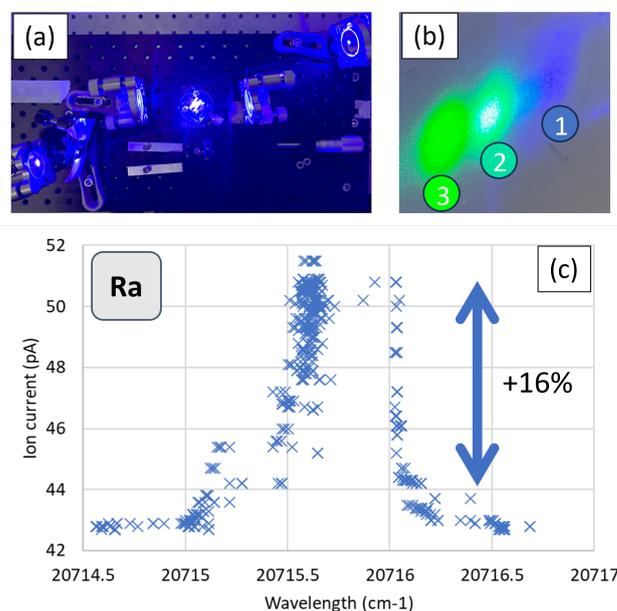
Figure 2: (a) Picture of the Raman laser z-fold design. (b) Generated beam from (1) blue pump (454nm), (2) 1st stoke (483nm), and (3) 2nd stoke (516nm). (c) First step laser ionization resonance of Radium using the Raman laser.
