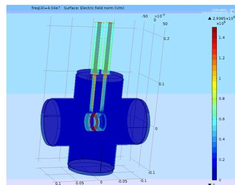
Figure 3: Electromagnetic study of the buncher system.
