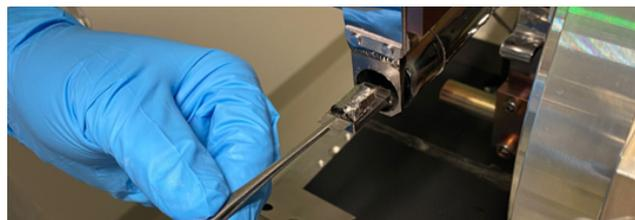
Figure 4: Ti sample being removed after release
