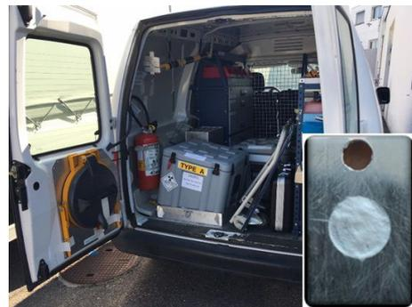
Figure 1: Road transportation with type A container containing  $^{149}\text{Tb}$  MEDICIS collection for delivery to CHUV; figure inset - salt coated aluminum foil.
