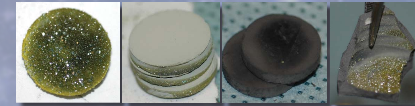
Material evolution of sub-micron SiC target after proton irradiation
