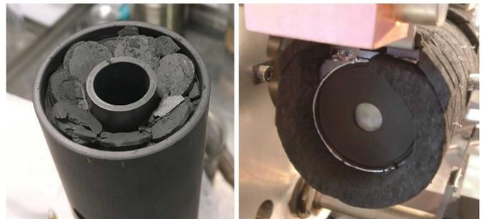
Figure 1: Left - filling of the graphite sleeve of the p2n-converter prototype with standard  $UC_x$  pellets; right - photo of the p2n-converter with special thermal shielding and target cap opened where the W bar can be seen inside of the  $UC_x$  containing graphite sleeve.
