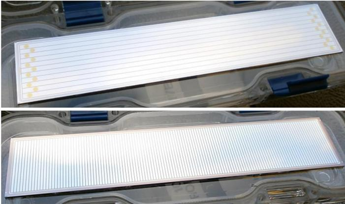
Figure 2: Photographs showing an ISS DSSD. In total 24 DSSDs with ASIC readout are required for the full ISS array.
