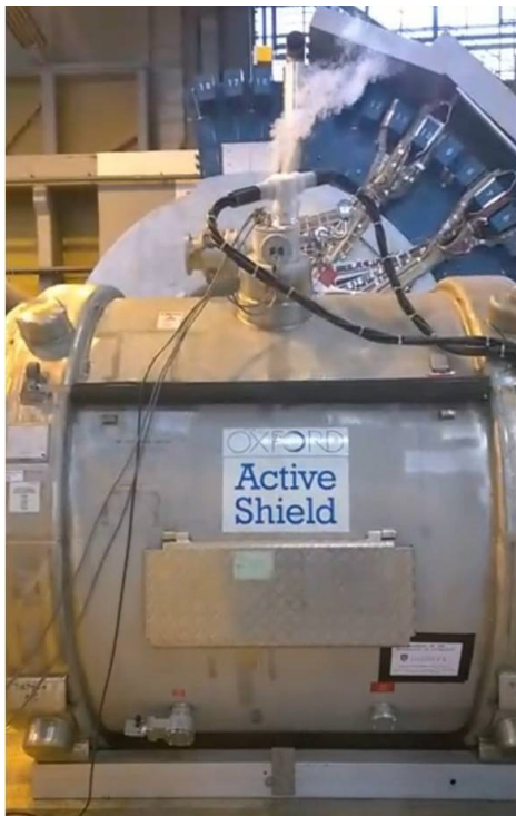
Fig. 1: Photograph of the ISS magnet during the energising procedure at CERN in February.
