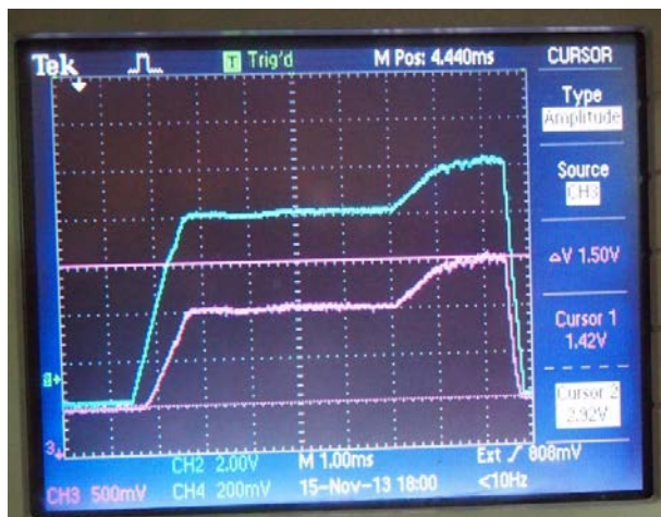
Fig.3: A 7 ms current pulse of at maximum 1.5 A (pink) extracted from the HEC 2 gun.
